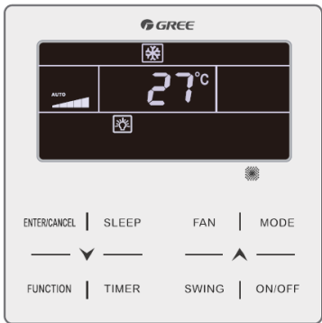
Fig. 4.1 Interface of On status
