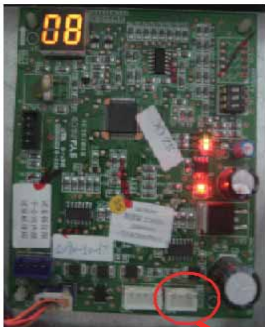
The patching board is not communicated with indoor unit ( Fig 1 )
