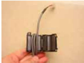
Fig.6.2.5.2 Connection Manner of Crystal Connector, Communication Line and Magnetic Ring
