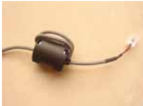
Fig.6.2.5.3 Connection Location of Crystal Connector, Communication Line and Magnetic Ring
