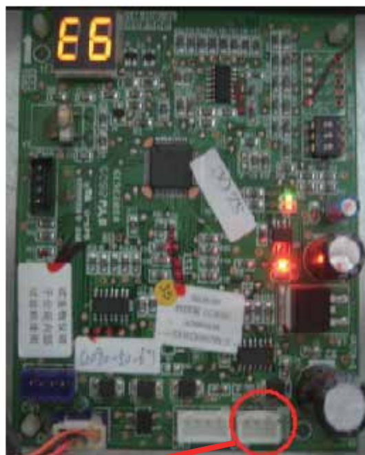
The patching board is not communicated with indoor unit ( Fig 1 )
