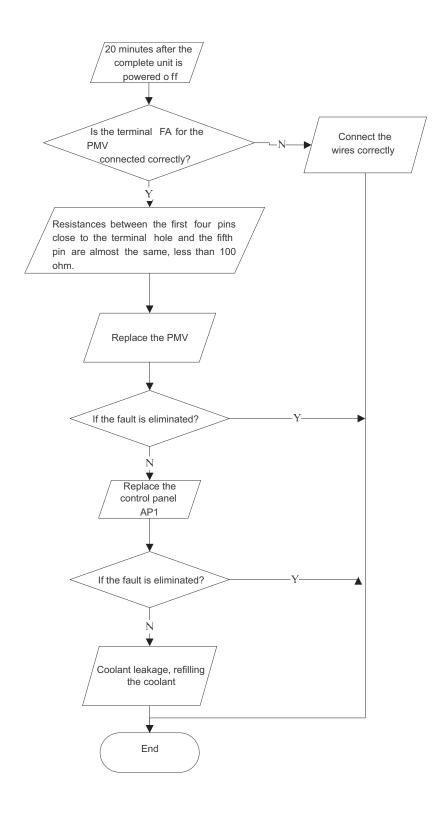
(7) Power factor correct or (PFC) fault (a fault of outdoor unit)(AP1 here in after refers to the control board of the outdoor unit)
