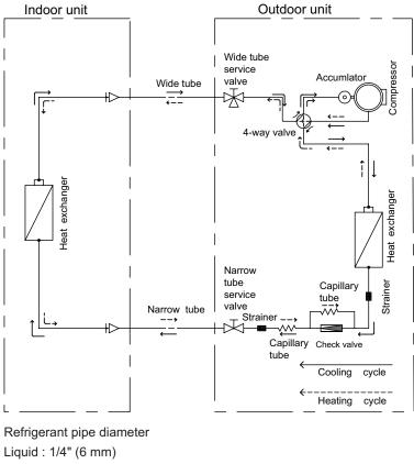
Liquid : 1/4" (6 mm) Gas : 3/8" (9.52mm)(09K) Gas : 1/2" (12mm)(12K)
