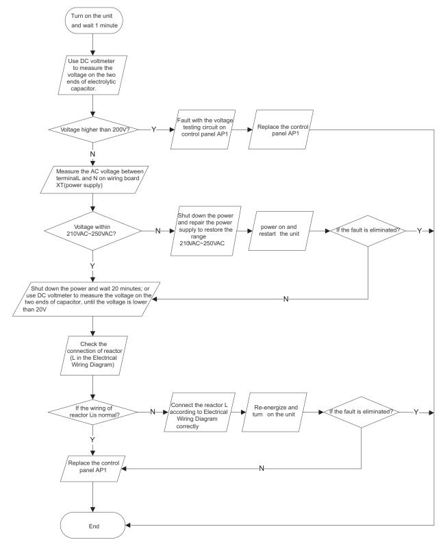
(2) IPM Protection, Out-of step Fault, Compressor Phase Over current(AP1 below refers to the outdoor control panel)
