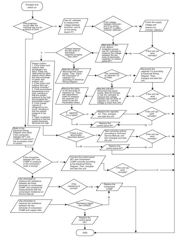
(3)High temperature and overload protection diagnosis (AP1 hereinafter refers to the control board of the outdoor unit) Mainly detect:
