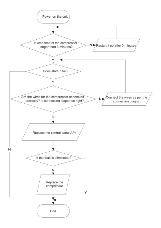
(5) Out of step diagnosis for the compressor (AP1 hereinafter refers to the control board of the outdoor unit) Mainly detect:
