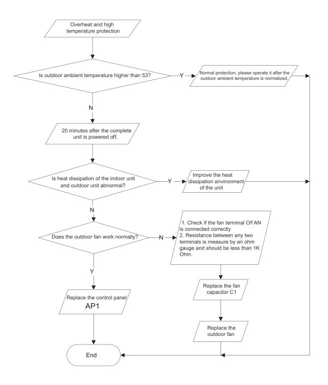
(4) Start-up failure(following AP1 for outdoor unit control board) Mainly detect:
